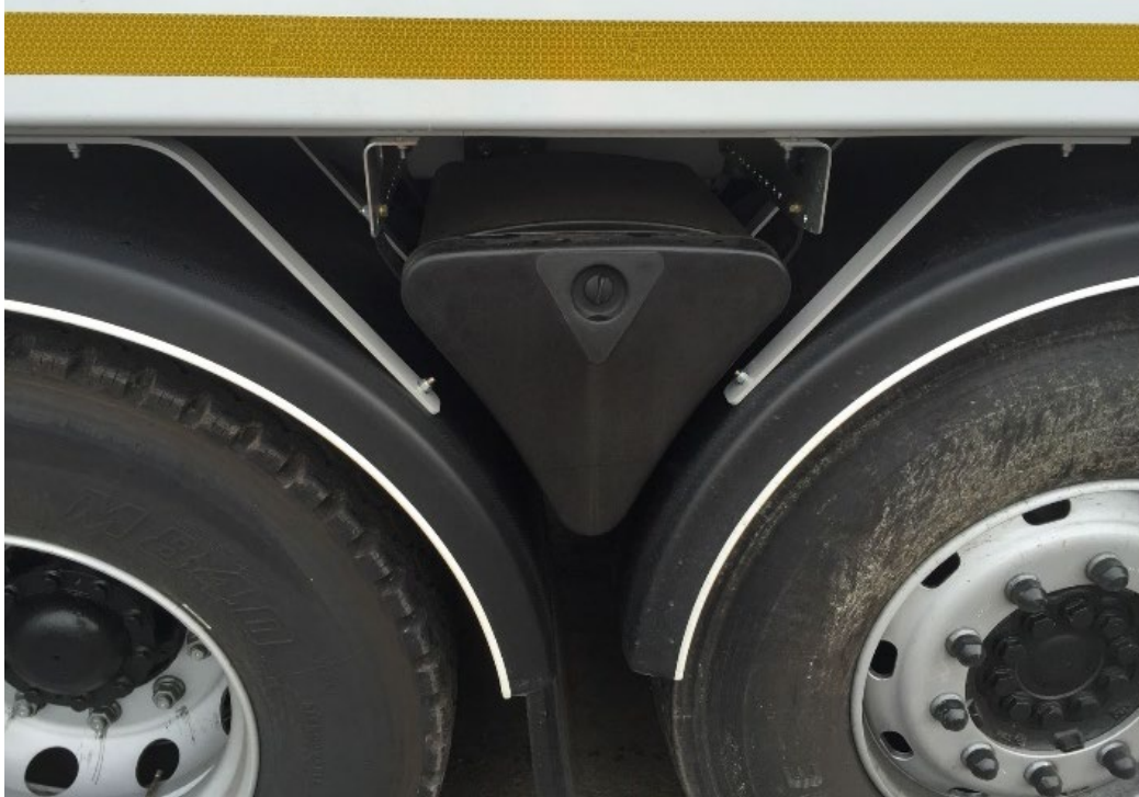
Figure 4 Example in Burnley where pods were fitted between wheels of the RCV for batteries.
