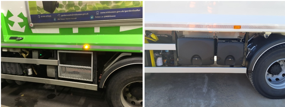
Figure 4 Example in Burnley where pods were fitted between wheels of the RCV for batteries.
